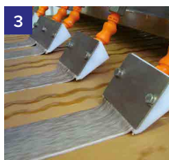
3 Creams or Jams distribution manifolds with specific design of the extruding nozzles
