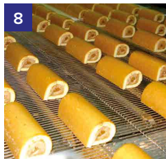
G-Tube Technology to bend sponge-cake and to fill it with creams
