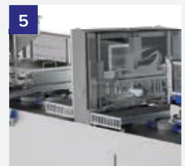
Pressing unit for crumbled with pneumatic pressing device
