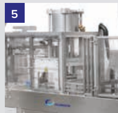
Pneumatic pressing device equippend with stainless steel heated head coated with teflon.
