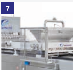
Volumetric doser machine Dosamatic or Dosatronic for jam, creams, fruit souce and chocolate
