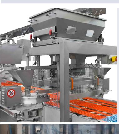
with ultrasonic guillotine system to divide into clear portions without dirtying or pressing cakes and can be equipped with printing systems with edible inks and robotic arms to decorate, write and replicate images, logos and more, to guarantee equal results on every single cake.
